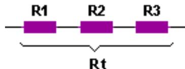
$$R_t = R_1 + R_2 + R_3$$
